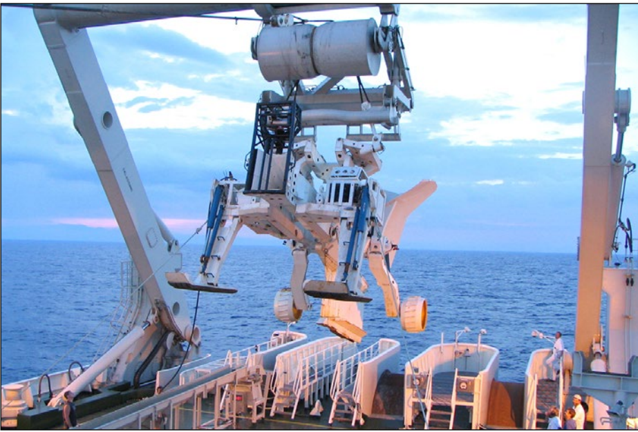
The sea plow, here ready to be launched from the ship, is used to dig a trench and bury cable in the ocean floor. An ROV then inspects and, if needed, completes burial.
